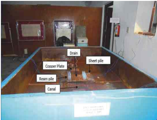
EHDA Model of Aqueduct at Km. 72.300 of Rapti Main Canal (UP) and Instrument Set-up in Ground Water Laboratory
