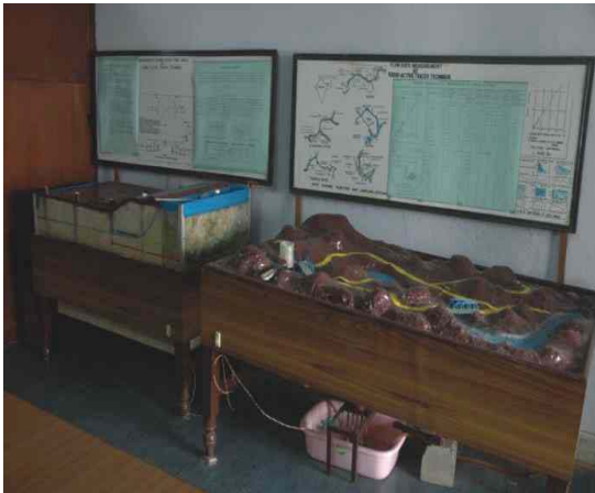
Models for measurement of Discharge & Seepage Laboratory Losses using Tracer Technique in Isotope Laboratory
